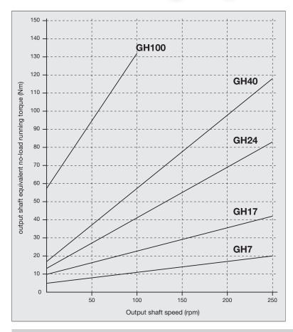
The no-load running torque that is converted to the input shaft side value should be calculated using the following equation:
