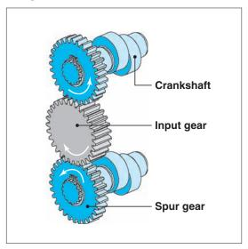
■ Fig. 2 Crankshaft section
