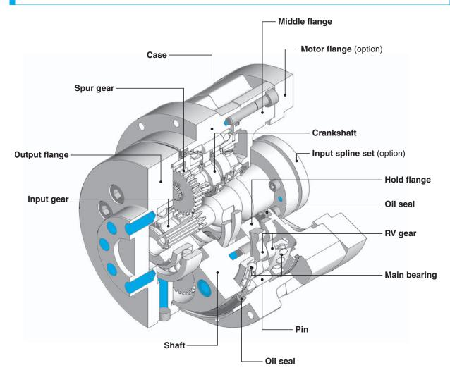
■ Rotation direction The rotation direction of the output shaft is same as that of the input spline.
